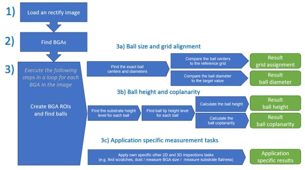
The image processing is performed with Halcon<sup>3</sup>. The sample code can be provided upon request to allow for fast start up and integration; however, other image processing libraries are also suitable to handle the data. This report is intended to show the general image processing procedure.
