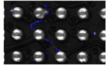
Green darkfield channel with edge detection filter function
