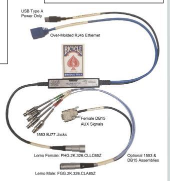
A/D Signal Capture Included on First Channel of NLINE. In-Field Signal Troubleshooting! Use AtaView or your Own Code to Scope/Compare Signals.
