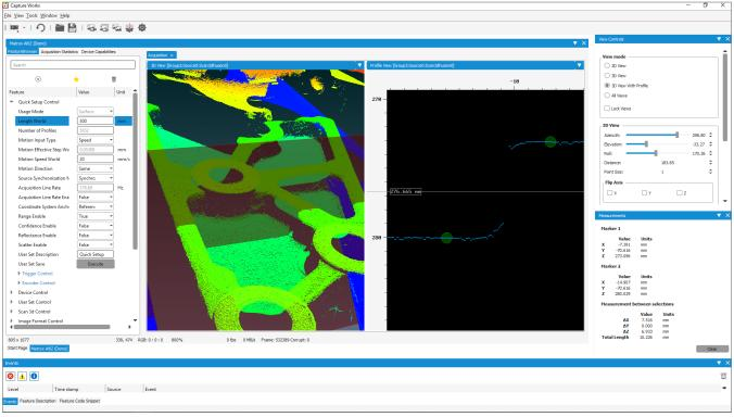
3D (point cloud) view with profile at intersecting plane and measurement markers within the Matrox Capture Works interactive utility.
