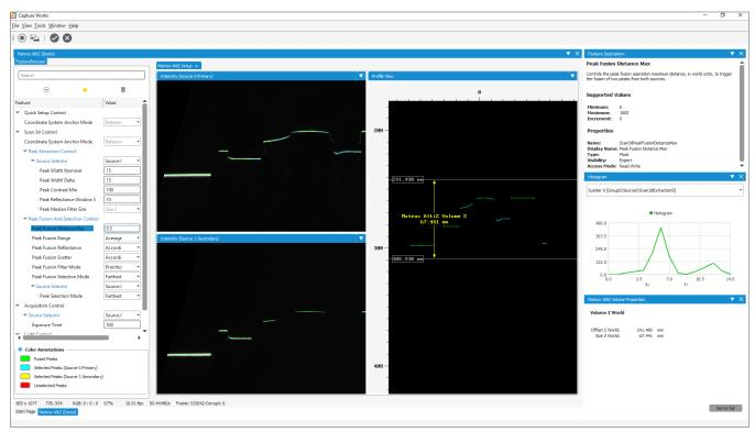
Peak (laser line) extraction, fusion, and volume (Z) adjustment within the Matrox Capture Works interactive utility
