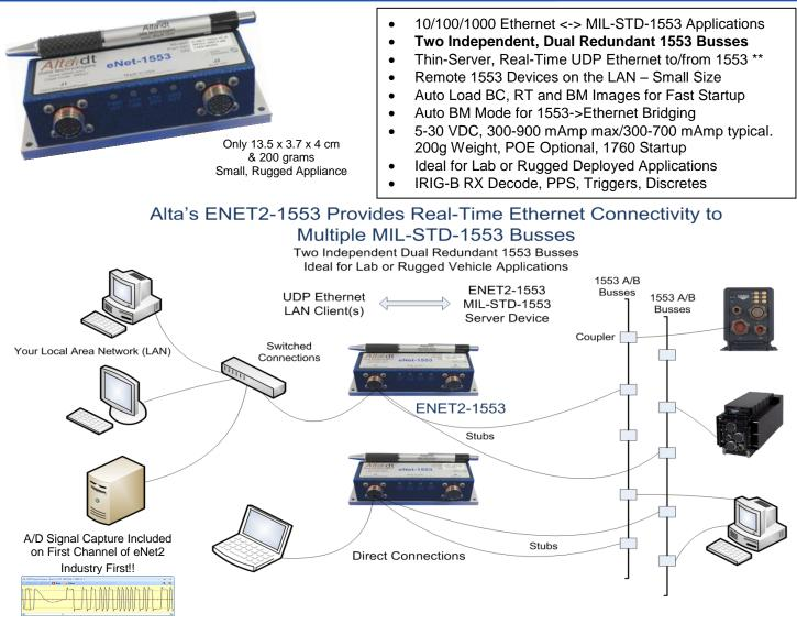
**eNet2-1553**<sup>™</sup> is an innovative product that provides "remoting" of 1553 operations on 10/100/1000 Ethernet IP/UDP local area networks (LAN). eNet2-1553 is a small, low-power, rugged device that provides real-time Ethernet connectivity to for **two** dual redundant 1553 (A/B) busses. Ideal for remoting 1553 connections for in-field applications or point-point lab usage.
