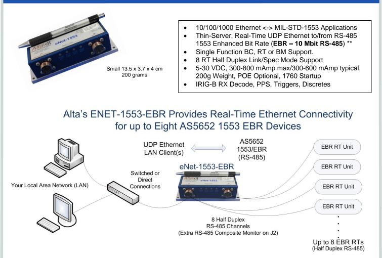
**ENET-1553-EBR**<sup>™</sup> is an innovative product that provides "remoting" of 1553 AS5652 EBR operations on 10/100/1000 Ethernet IP/UDP local area networks (LAN). ENET-1553-EBR is a small, low-power, rugged device that provides connectivity for up to eight AS5652 RT devices, single BC or composite monitor.
