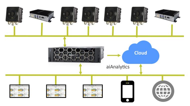
aiAnalytics is a turnkey solution for collecting and analyzing vision data from a large number of standard 2D & 3D vision systems. It easily connects to existing vision systems using a variety of interfaces to gather part inspection, metrology, image, & point-cloud data. This data can be explored from any location using desktop, web, and mobile application.
