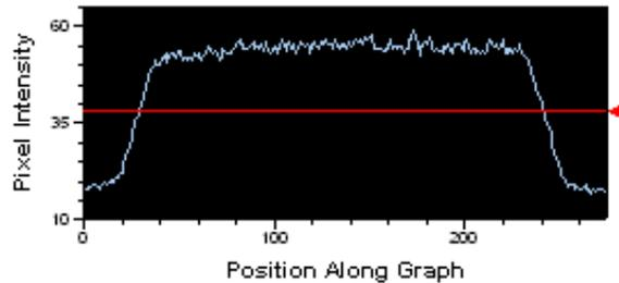
The LLPX offers a very diffuse light pattern at any defined working distance. The Pixel Graph representation shows a steep drop off in intensity outside of the active area with a very diffuse light pattern inside.
